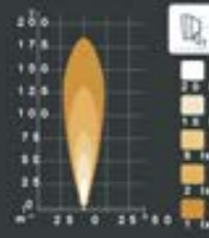
High Beam projected on surface #A
