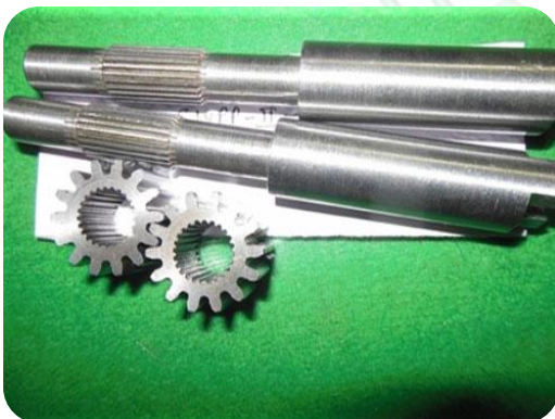
External Splined Shaft with matching gear (internal Spline) ( Module : 0.25)
