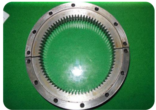
Internal gear with module 0.5 in two halves
