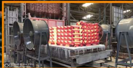
4 NOS (10 TON / 5 TON / 5TON / 1 TON) HEAT TREATMENT FURNACE WITH AUTO CONTROL WATER & AIR QUENCHING FACILITIES
